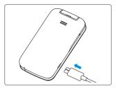
Insert the small end of the charging cable into the charge port as shown and connect the charger to a power outlet.
